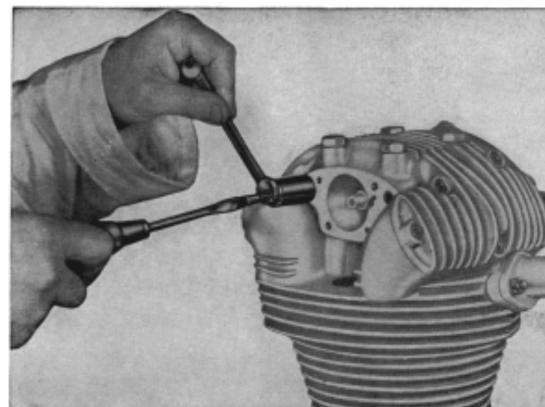
11 - Extractor for rocker pin
