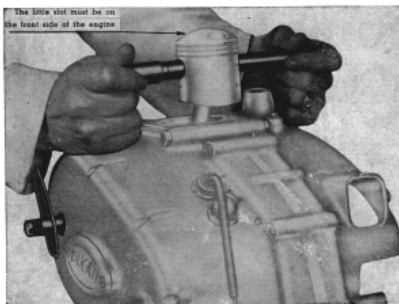
16-17 - Pins to fit and re-fit gudgeon pin
