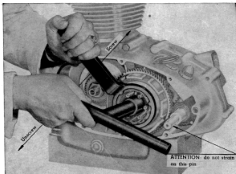
5) Spanner to secure the clutch drum
