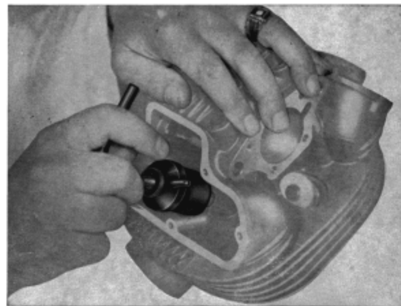
8 - Clamp for lapping the valve seats
