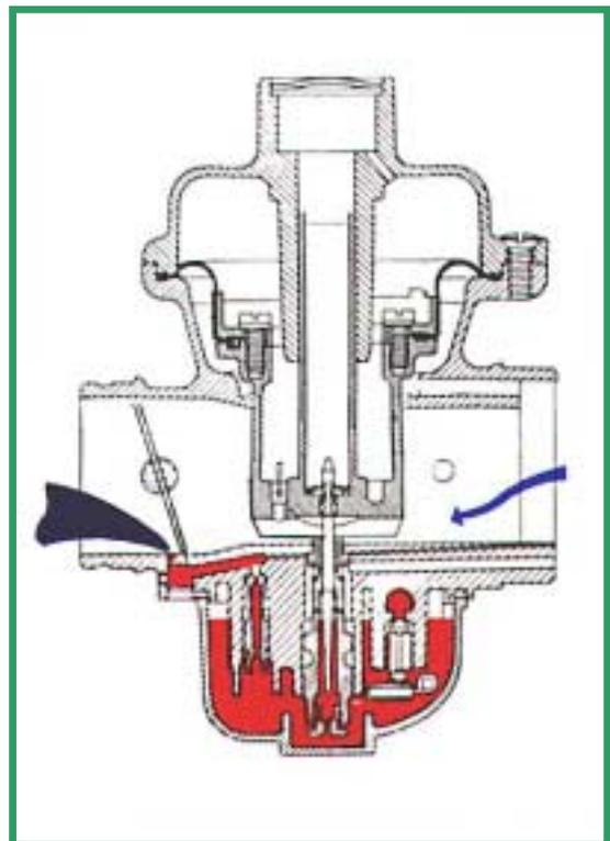
CV carb has no accelerator pump. Accelerator pumps generally provide a brief mixture enrichment during sudden throttle openings for increased power and hence acceleration. They are usually mechanically operated rather than vacuum operated. But the principle of the CV carb produces an effect very similar to that of the more traditional pump.
